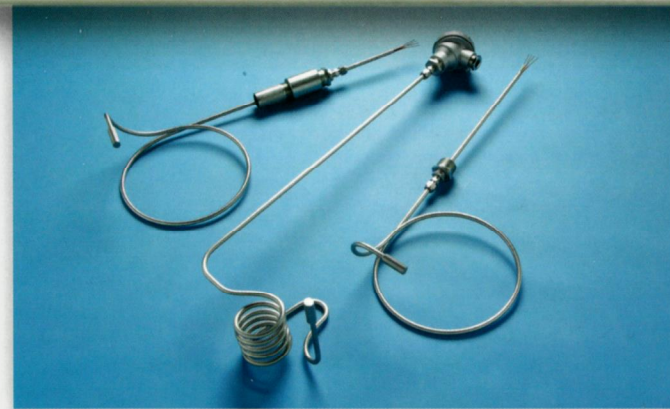
Miniature, superfine thermocouples are available for fuel cells, medical research and other applications where space is limited. Sheath diameters start at 0.004" with bare leadwire, potting adaptor or miniature plug connector styles offered.
