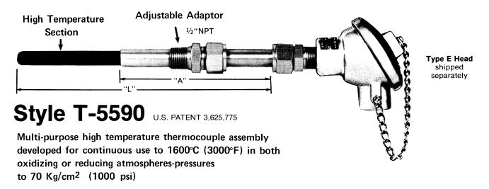
HIGH TEMPERATURE SECTION: 12.7 mm (0.5 in.) diameter LENGTHS FROM 76.3 to 433 mm (3 to 17 in.)
