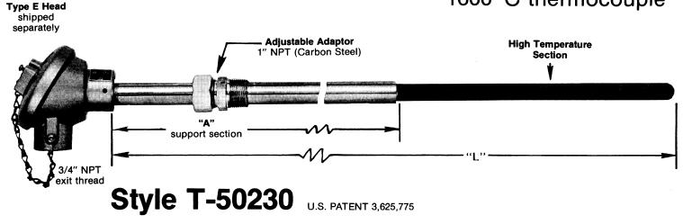
HIGH TEMPERATURE SECTION ("L"-"A"): 19mm (.75") diameter cermet well to 430mm (17") long
